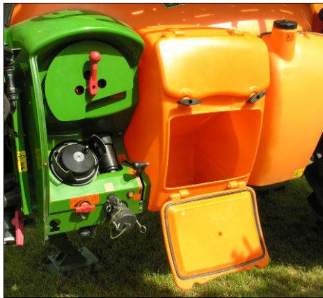
Figure 69: The high capacity locker for the hose of filling device to protect it from contamination
