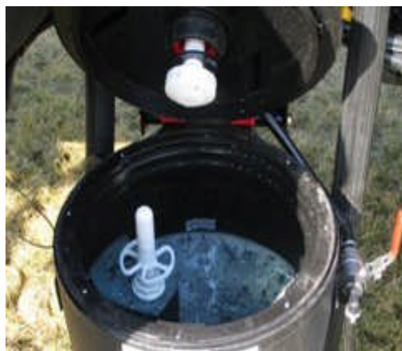
Figure 29: Rinse nozzles for induction hoppers allow safe cleaning of internal surfaces.
