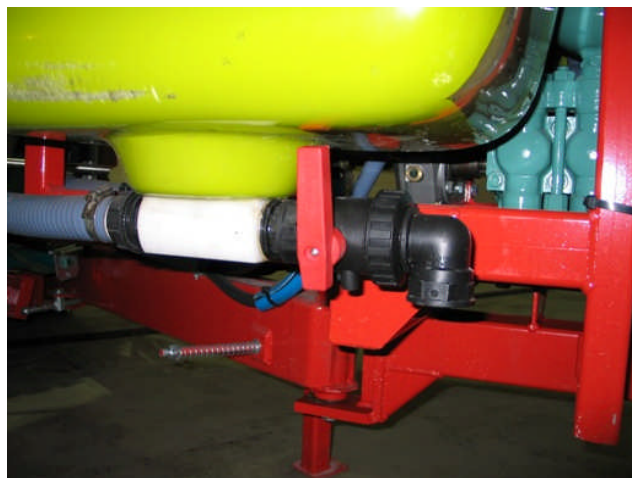
Figure 101: Sump at tank bottom
