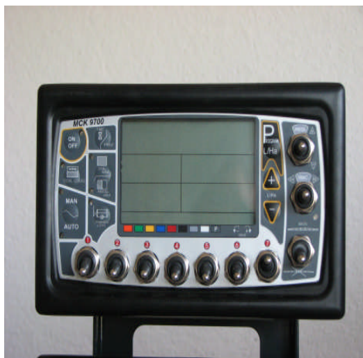
Figure 94: Electric ON/OFF valves operated from the tractor cabin.
