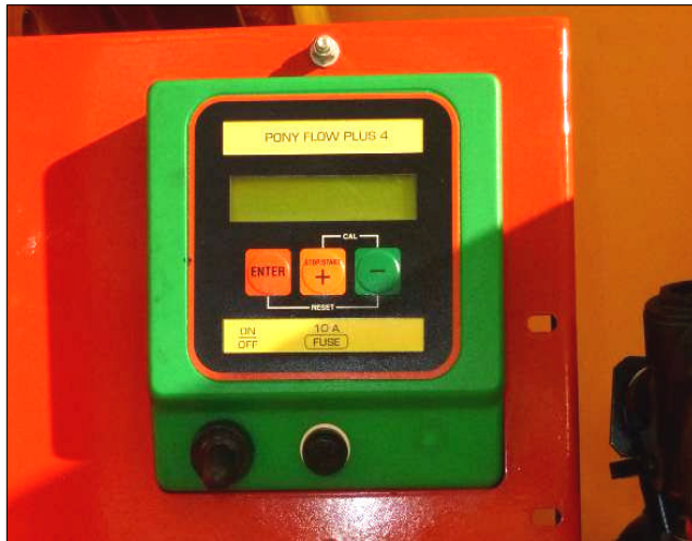
Figure 80: Programmable flow meter to control the volume of water filled to the sprayer tank
