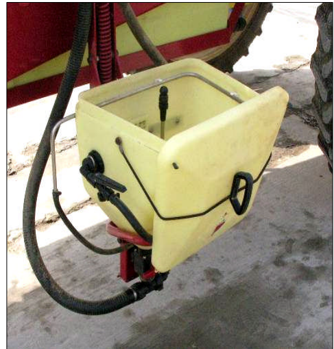
Figure 60: The contaminated liquid may drip from the induction hopper's cover attached loosely by string or chain
