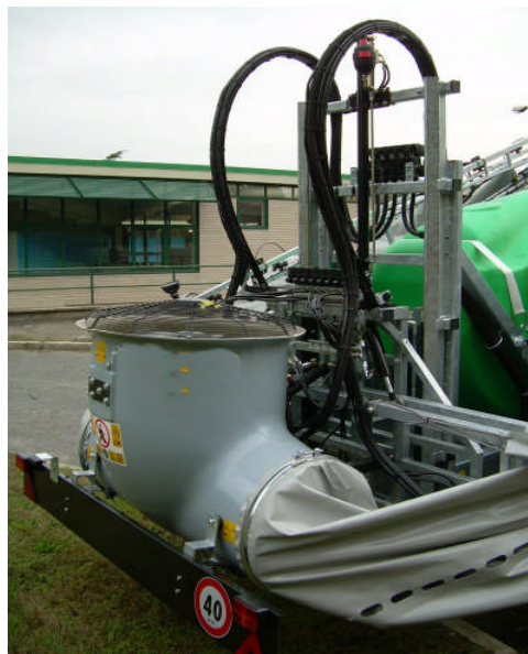
Figure 124: Hydraulically driven fan on a boom sprayer.
