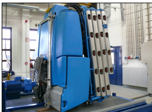
Figure 42: Shielded, smoother lined, sprayers are more easy to clean
