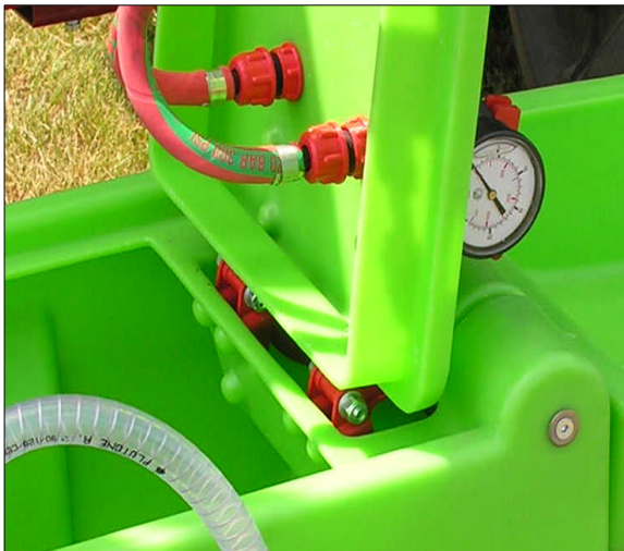
Figure 59: Induction hopper's cover attached by hinges eliminates the risk of spillage
