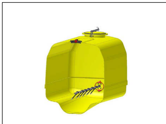
Figure 27: Rinse nozzles mounted on a rotating axle that can effectively reach all inner tank surface using high speed impact water jets
