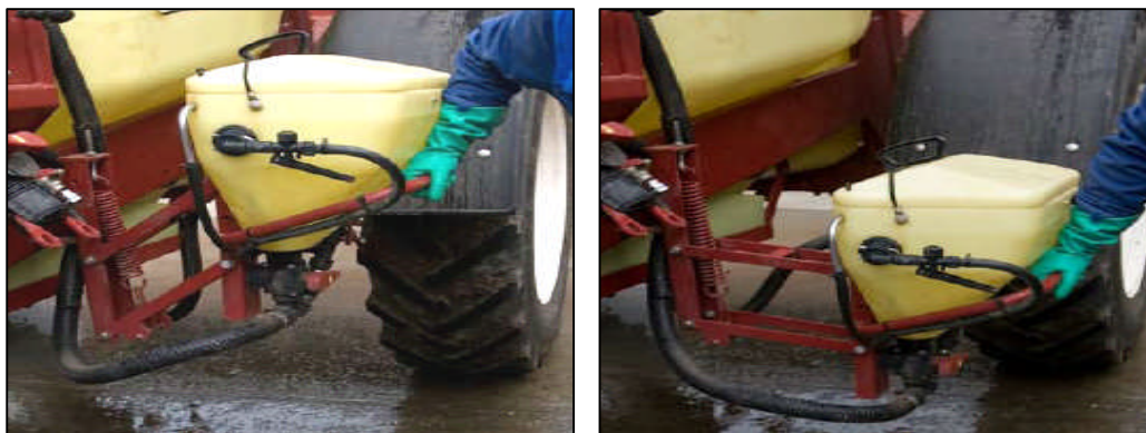
Figure 54: Induction hopper assembled on a folding system for lowering to the convenient working position
