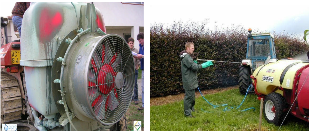
Figure 15: PPP deposits on sprayer outside and cleaning device attached to the sprayer to enable field cleaning from outside.
