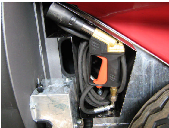
Figure 45: Device for external cleaning protected behind a cover
