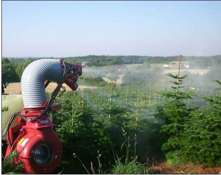
Figure 111: – Cannon sprayer creating spray plume at long distance and therefore prone to drift
