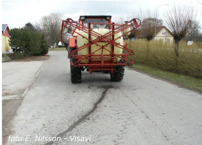
Figure 132: A leaking / dripping sprayer during its transport from the farm to the field.
