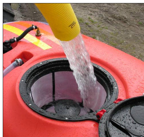
Figure 66: Deep strainer facilitates safe and efficient filling of the tank with water with no risk of splashing
