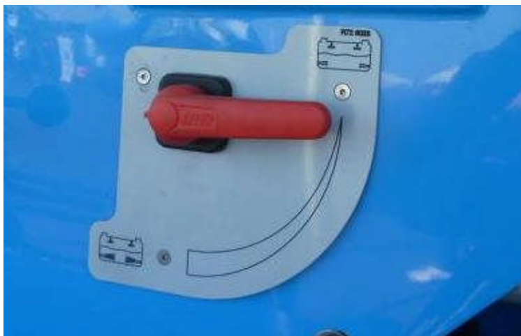
Figure 34. Turning off agitation- when main tank volumes of PPP solution are low - reduces the retained residual volume.
