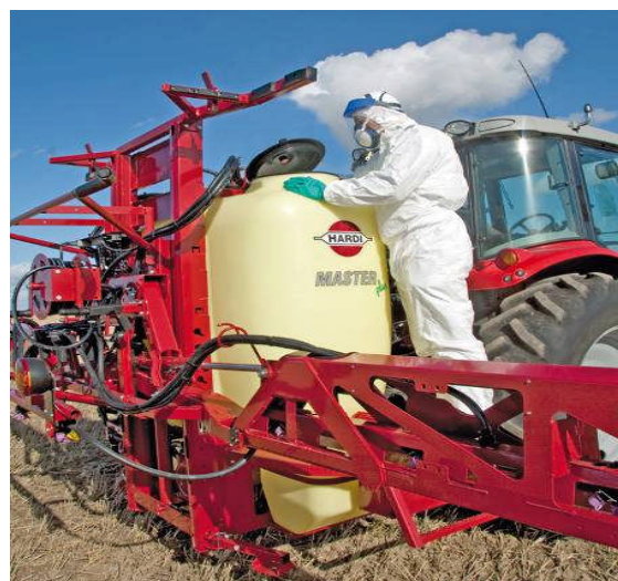
Figure 65: Asymmetrically located filling hole makes it easily accessible by the operator
