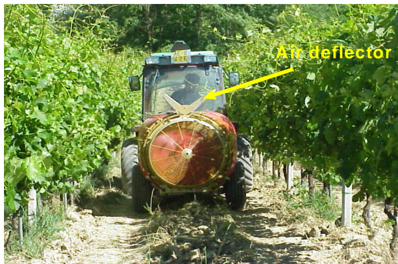
Figure 126: Air deflectors to be adjusted manually on a vineyard sprayer
