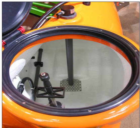
Figure 64: Filling hole diameter should be large enough to facilitate an intensive flow of water with a minimum risk of splashing
