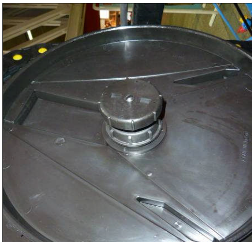
Figure 82: Air valve for pressure compensation in tank
