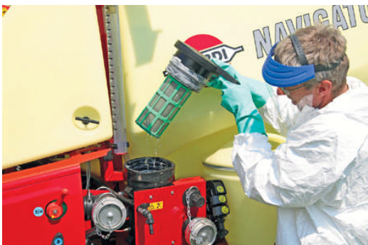
Figure 36: Vertically positioned filters allow the opening of the filter house without spills
