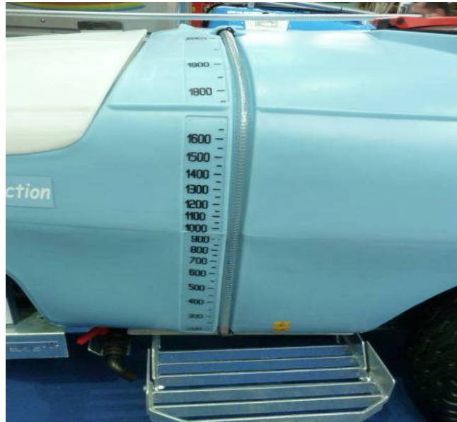
Figure 79: Tank of nominal volume 2000 l with a liquid level indicator with scale interval
