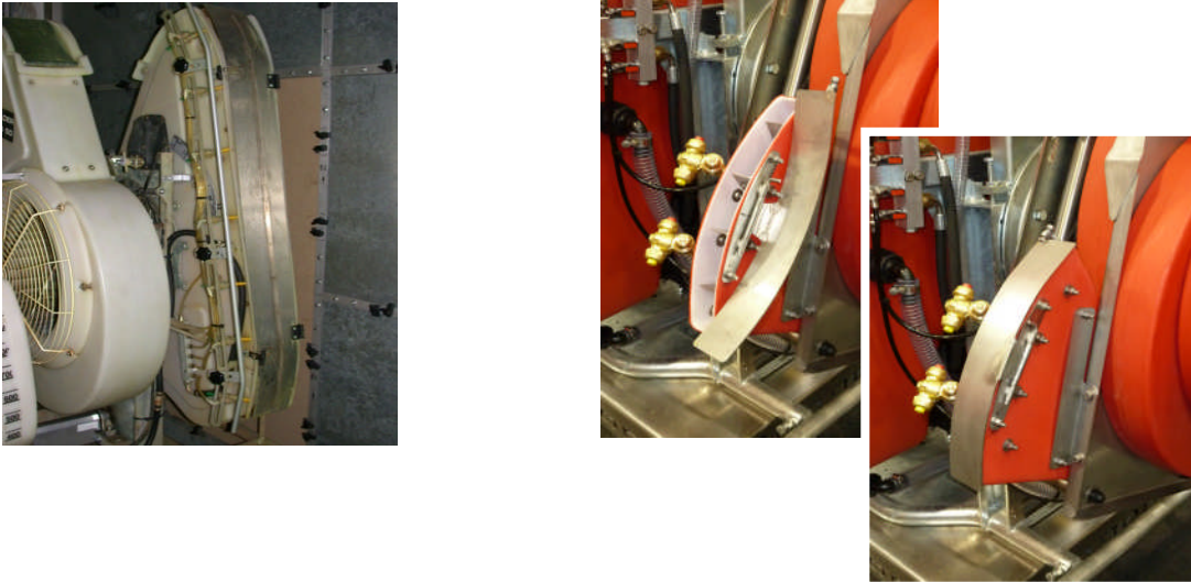
Figure 125: Covering systems on air outlets of orchard sprayers to close the airflow on one side of the sprayer
