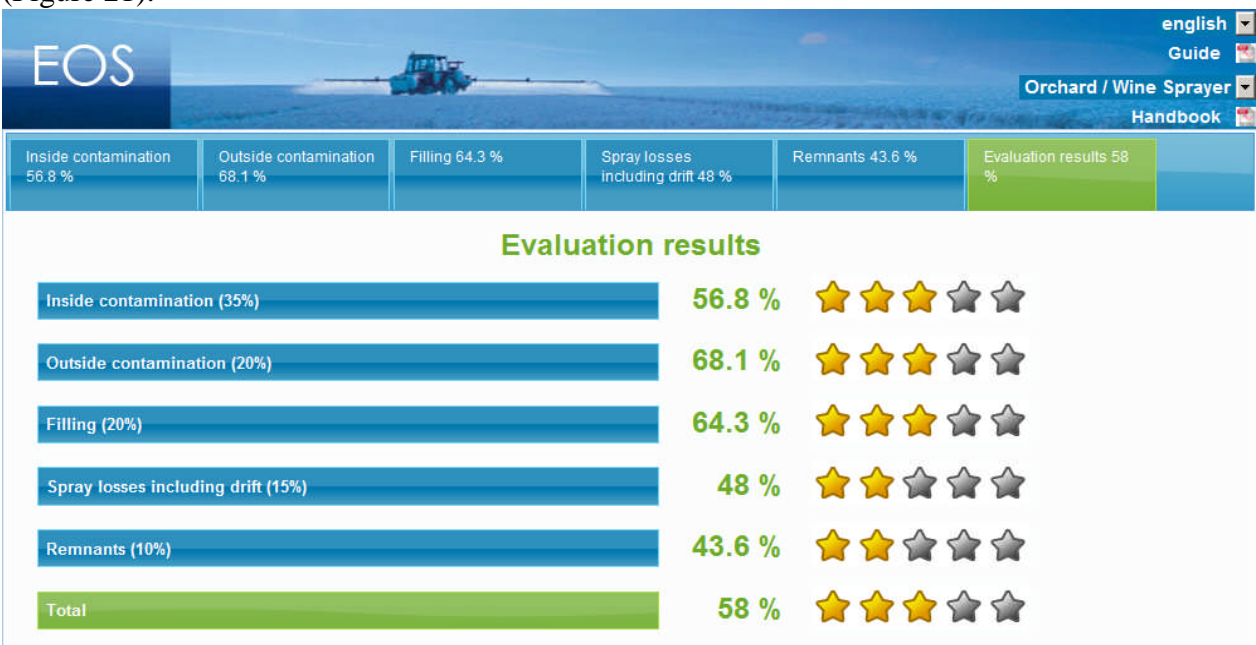
Figure 21: Display of evaluation results after completion of the EOS questionnaire. EOS index expressed in %, stars will indicate the rating of the sprayer.
