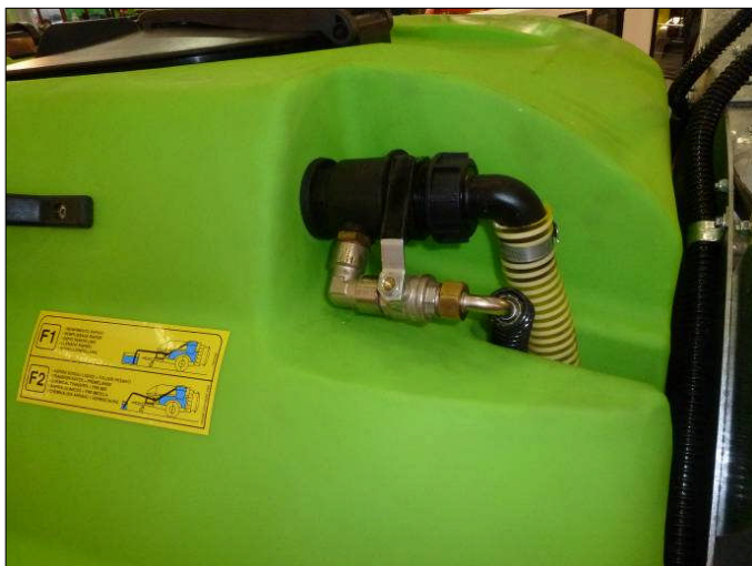
Figure 51: Injector for inducing the PPPs from the container to the sprayer tank
