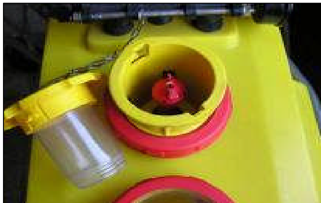
Figure 55: Antispill opening on the cover of induction hopper for safe introduction of PPPs
