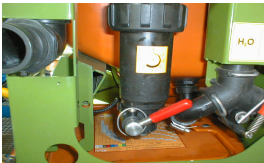
Figure 37: Self cleaning filters in pressure lines reduces maintenance checks on other filters and nozzles
