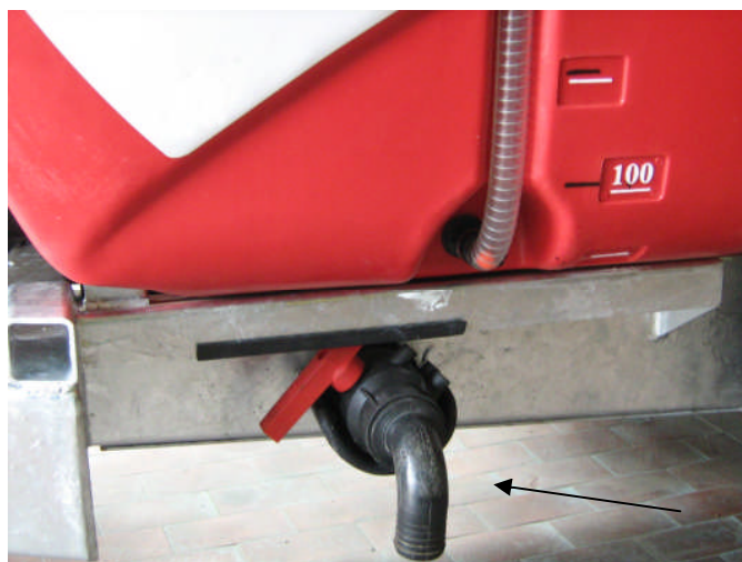
Figure 98: Drain valve positioned at the bottom of the tank. (an EOS sprayer should allow the safe and complete emptying of the complete sprayer)
