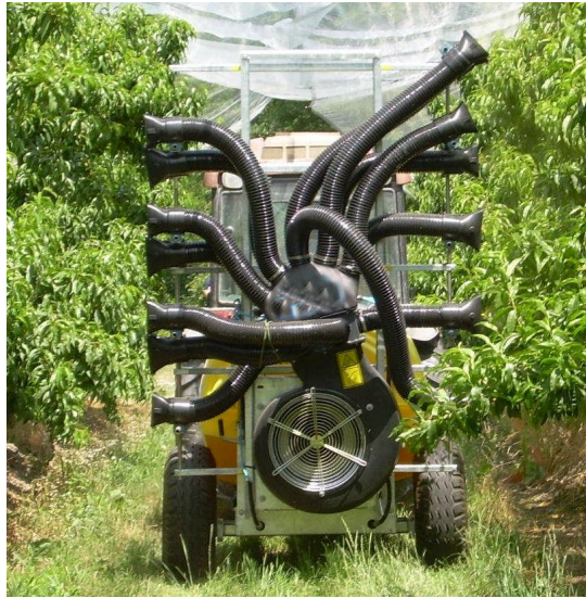
Figure 113: Directed air jet sprayer equipped with multiple and adjustable air spouts, each provided with nozzles.
