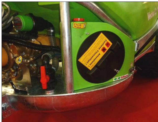
Figure 84: The lockable PPP locker retaining spills
