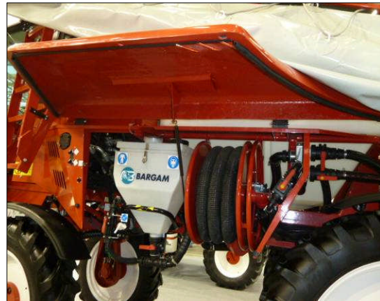
Figure 70: The hose of filling device covered to protect it from contamination
