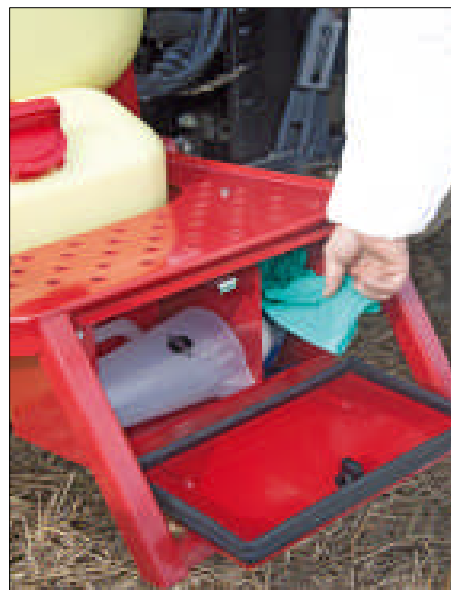
Figure 88: The dose measuring devices should be transported in a locker able to retain spills
