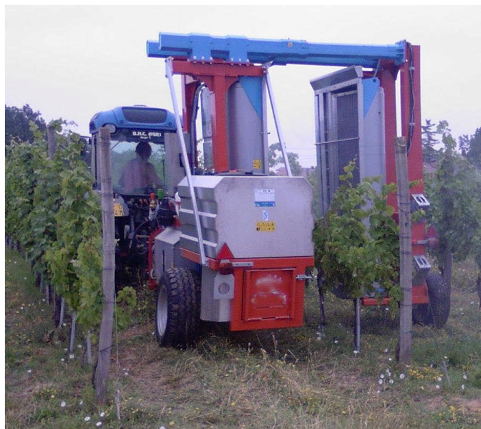
Figure 114: Tunnel sprayer generating spray plume roughly confined to the target size and collecting part of not deposited spray for recirculation
